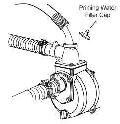
IMPORTANT! Always check for water in the Pump Housing before each use. Never attempt to run the Water Pump without the Pump Housing FULL of water. Running the Water Pump without water for an extended period of time will damage the Water Pump and void the Warranty.
